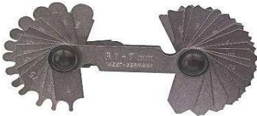
A photograph of a set of radius gauges, which are precision measuring tools used to measure the radius of concave or convex surfaces. They consist of a central stem with a dial gauge and two adjustable jaws with serrated edges. | 2 sets | 2 sets  |
